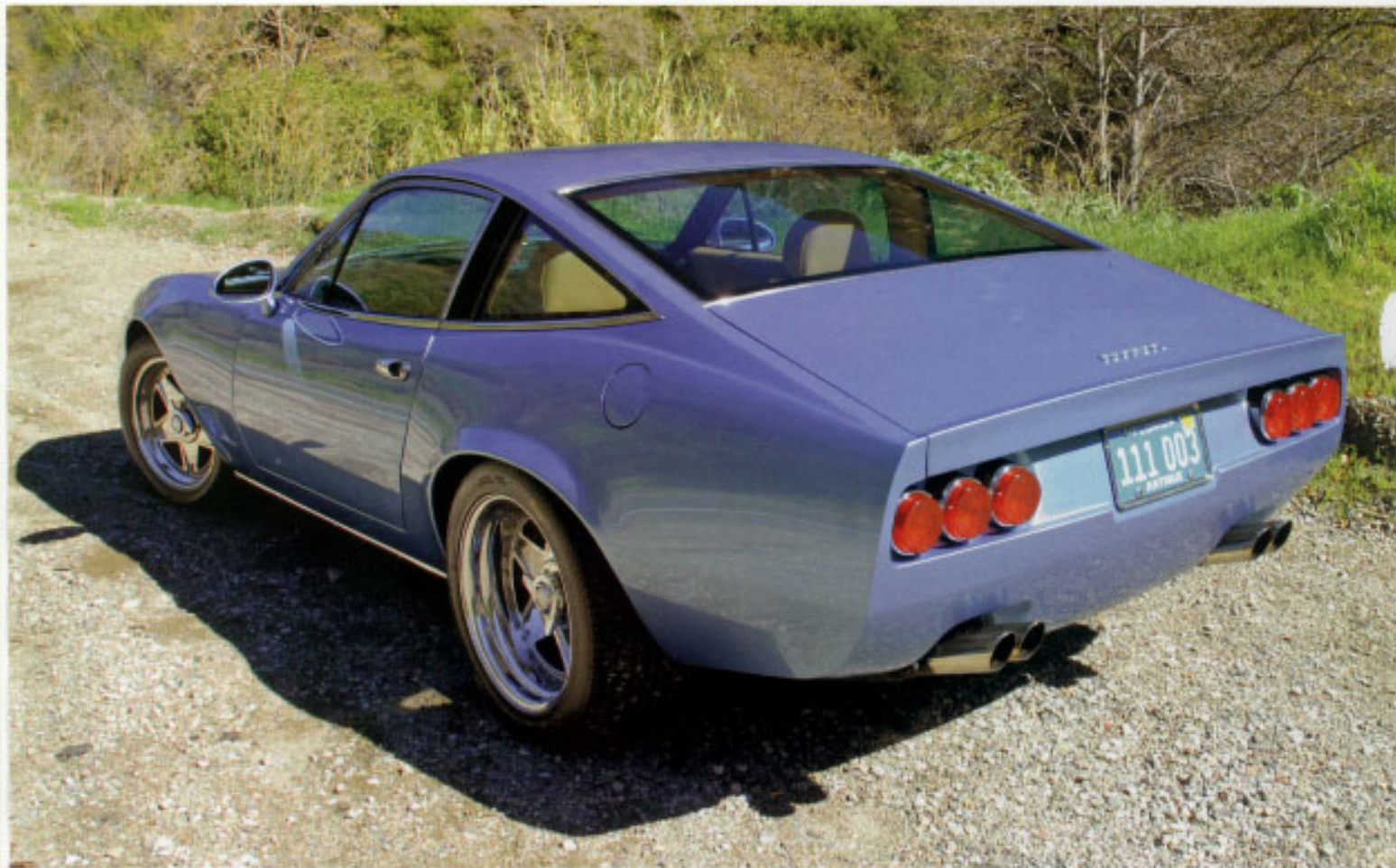
Above: Customized rear end features widened fenders, bumperless butt and subtle decklid spoiler. Left: New interior furnishings include 550 seats and reworked door panels. Below: Parcel shell replaced rear seats.
